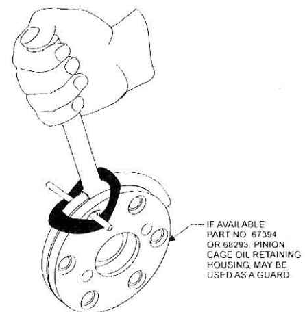
Figure 4. Crankshaft Propeller Flange Showing Installation of Stretch Seal Using a Guard Over the Front of the Flange
